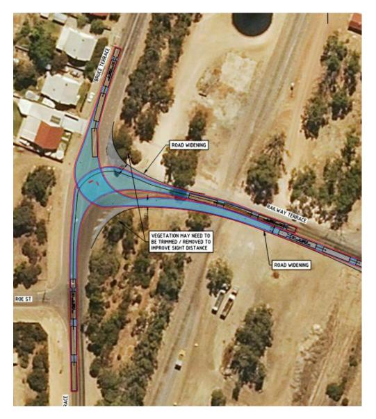
Figure 25 Concept Layout – Viterra Access Option 1
