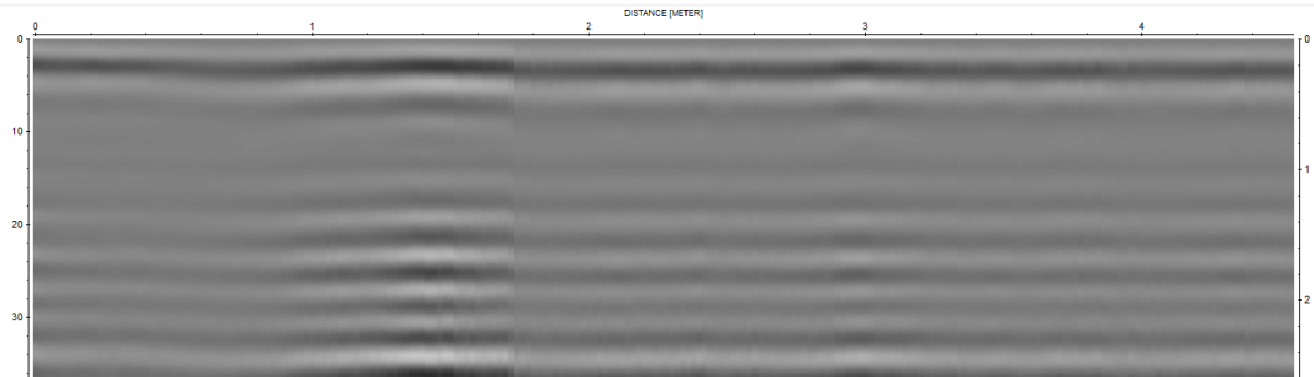
Figure 5: Example of GPR trace from Grid 3. This is indicative of all traces along Pine Grove Rd.
