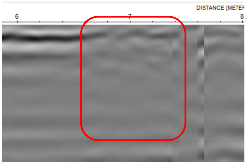
Figure 6: Example of GPR trace with shallow disturbance.
